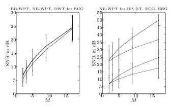
Fig. 1. Left: rate-distortion curves for BB-WPT, NB-WPT, and DWT compression of ECG; Right: NB-WPT compression of BP, NT, ECG, and EEG; both in decreasing order.
