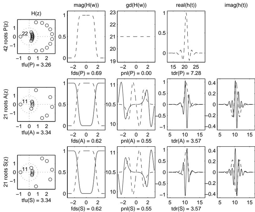
Figure 2: Daubechies Complex Orthogonal Most Symmetric DCOMS(22;11).
