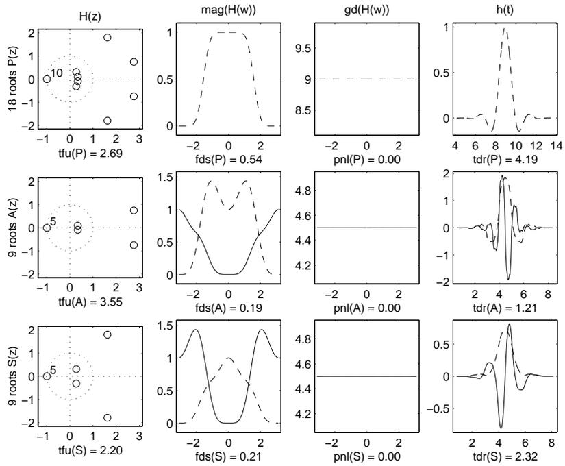
Figure 1: Daubechies Real Biorthogonal symmetric balanced Most Regular DRBMR(10,10;5,5).
