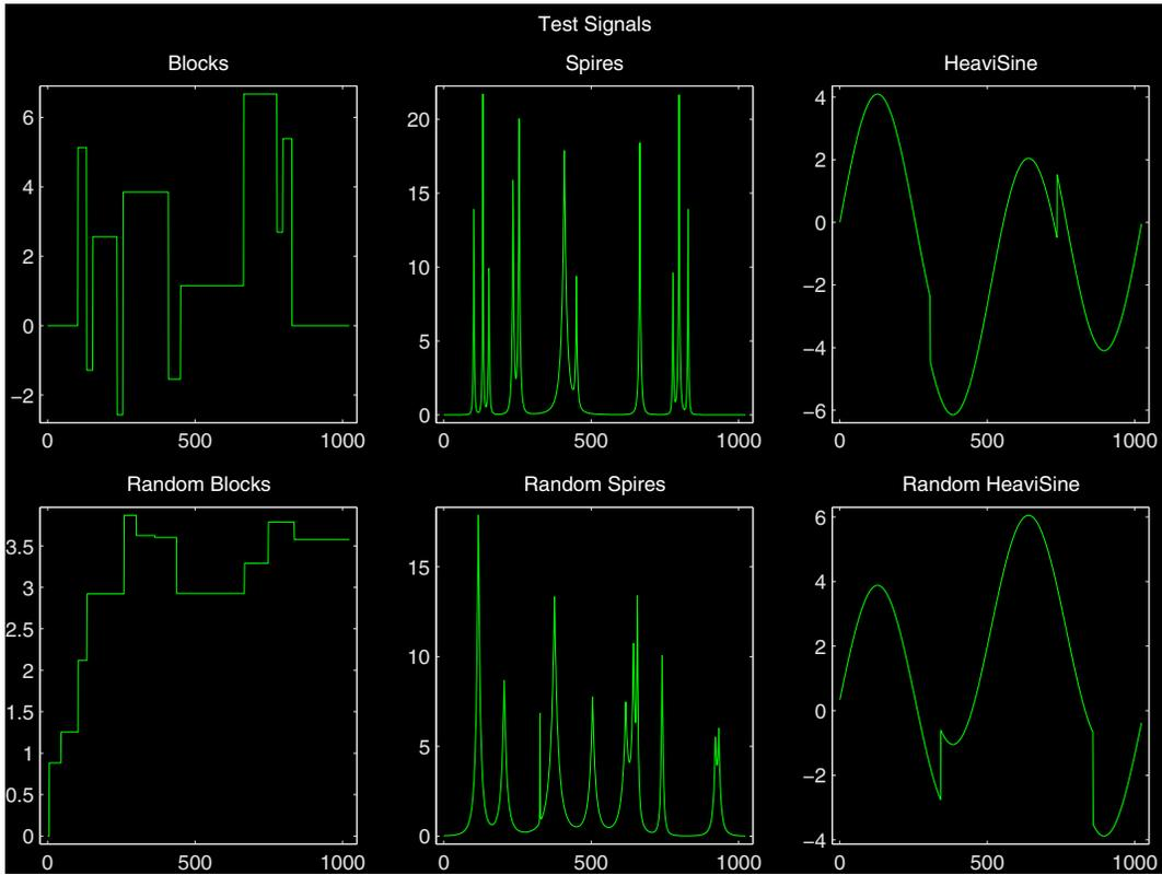
Figure 1: Standardized Test Signals.
